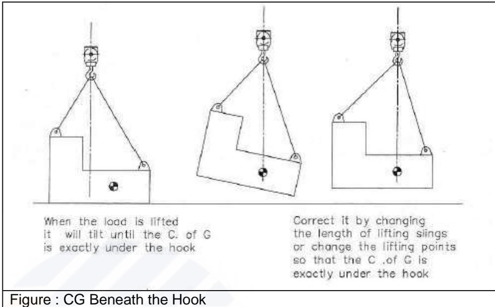
With larger and off-set/off balanced loads the CG is more difficult to determine. Below is an example of a load with an off-set CG. Normally this is the case at non symmetric elements. Note the slinging arrangements and how a load becomes unstable when the CG is not directly below the hook block.
