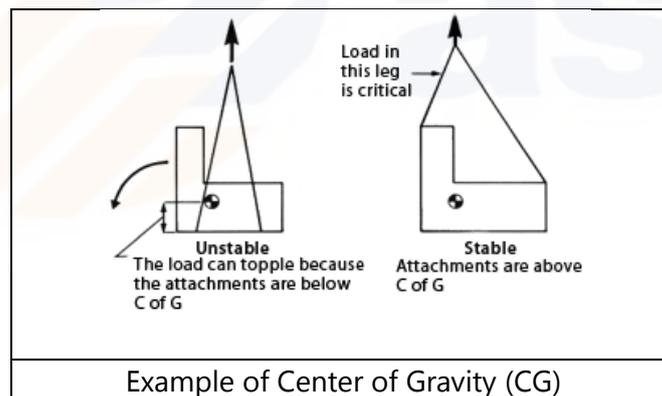
Note: For large objects which are being lifted, the CG. will have to be determined via engineering method. The lifting lugs will also need to be designed for to ensure safe lifting. Specific lifting gear can also be used to ensure that the hook is always above the CG during the lifting operation.
