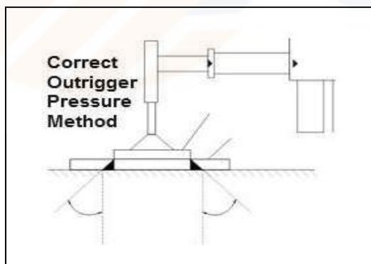
All normal routine & non-routine lifting operations with hydraulic mobile cranes must have outriggers fully blocked out using appropriate load bearing mats.
