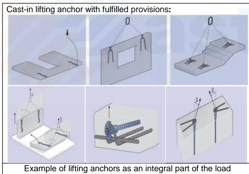
There will be cases where lifting lugs/pad-eyes will not be provided separately, but self-produced in the precast yard. In such cases the Engineer / Competent Person must be sure that they have current certification and are of sufficiently designed and verifiable proven to cope with the lifting effects.
