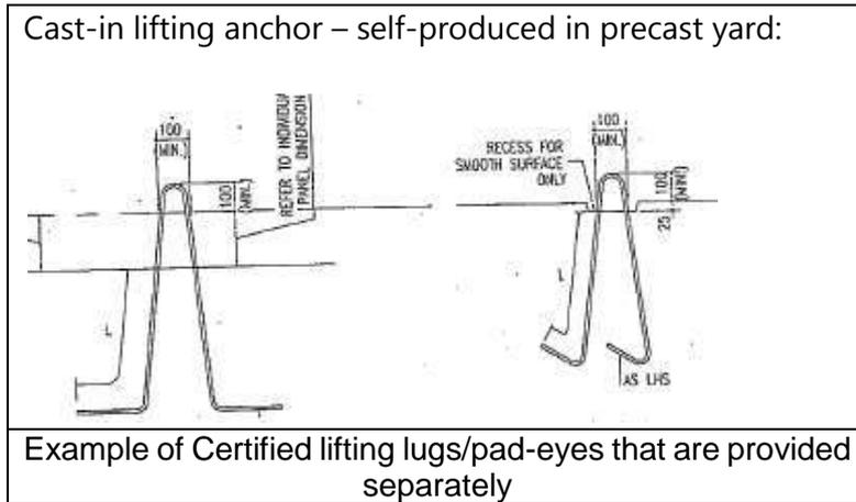
To avoid any risks for human life and health and safety of employees in the precast yard and construction site all lifting anchor systems and motions therewith have to be checked, calculated and proven by an constructional engineer e.g. as consultant or technical engineer in the precast yard. The resistance comes from supplier. In case of a given recommendation provided by supplier, the responsible engineer has to check the complete situation of handling too.
