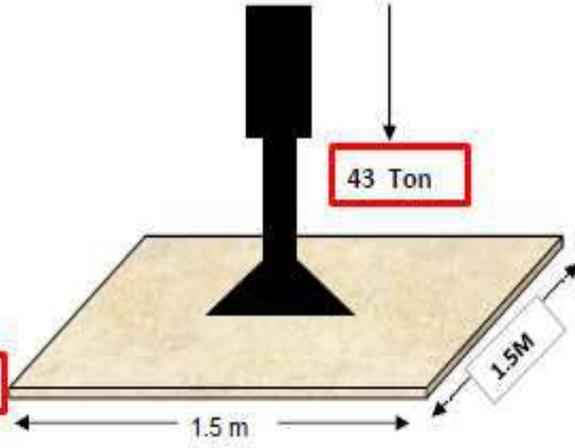
Example of Calculation for Ground Bearing Capacity
